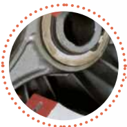
Needle bearing in both connecting rod eyes
